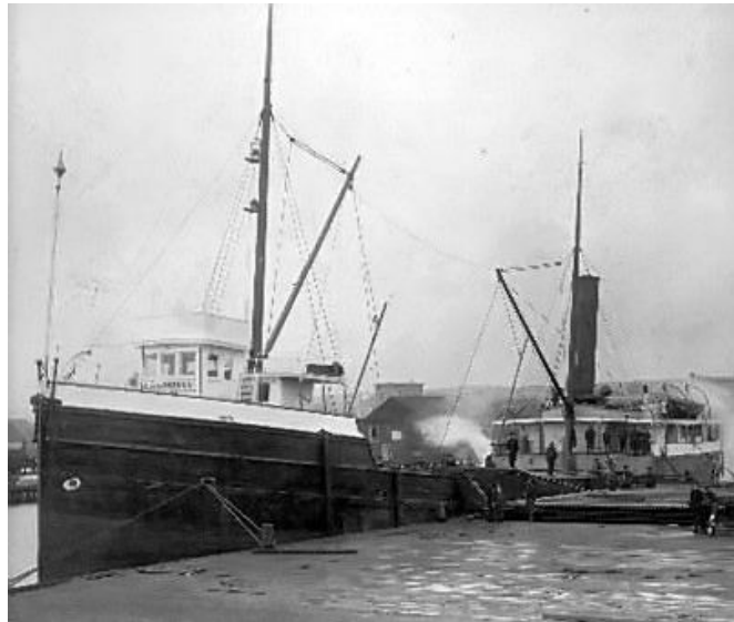
Turn of the 20 th century, steam driven, bulk cargo canal boat, unloading at Port Arthur. Wheelhouse is forward, the engine room is aft. This boat has a wooden hull, and the DUNELM's was steel.
